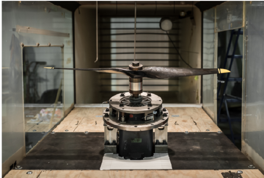
Figure 4 Rotor a un ángulo del eje de -14. Recuperado de Isolated Rotor in Forward Flight Testing From One Atmosphere Down to Martian Atmospheric Densities by Ament and Koning
